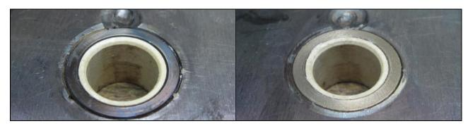
No measurable diameter reduction could be found on the plastic shaft. The smooth running tracks can be seen in diagram 3.
