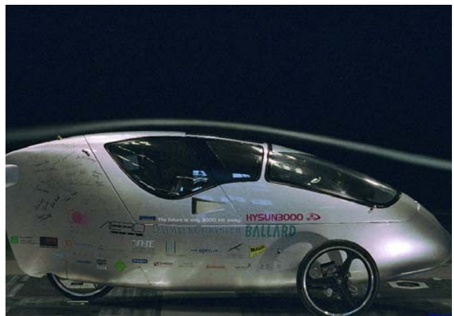
Bild PM1205-05: ExtraEnergy e.V., Kirchheim/Teck World-record breaking drive through Europe: The hydrogen-powered HYSUN3000 with joint heads and plain bearings made of plastic. Three times as many applications as in 2003 were entered for the "manus - 2 nd competition for plastic plain bearings". At the Hanover Fair, prizes were awarded in public to the winners, with the ceremony combined with a customer party.
